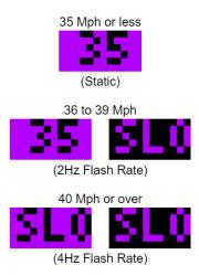
**Note:** "35" is not the vehicle's current speed, but rather the target speed. The alternating "SLO" is information for the driver to slow their car. Alternating "35 (black)/SLO (purple) indicates that a driver is within 4 mph of the 35 mph target. Alternating SLO (black)/SLO (purple) letters indicate a speed greater than 40 mph.
