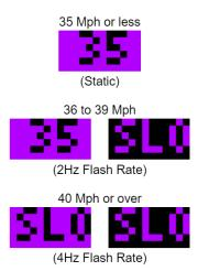
**Note:** "35" is not the vehicle's current speed, but rather the target speed. The alternating "SLO" is information for the driver to slow their car. Alternating "35 (black)/SLO (purple) indicates that a driver is within 4 mph of the 35 mph target. Alternating SLO (black)/SLO (purple) letters indicate a speed greater than 40 mph.
